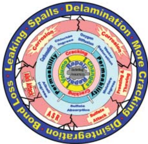
Fig. 2: Idealized model of repair failure
